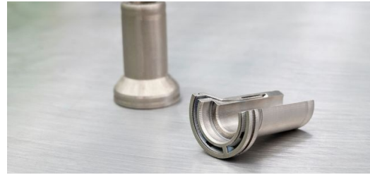
Amorphous metals are produced by flash-freezing molten metals. The atoms solidify in a random arrangement and do not form crystal structures.
