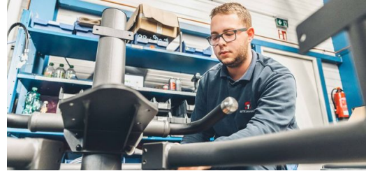
The frame of an EGYM exercise machine consists of primarily oval steel tubes. After processing on a TRUMPF laser tube-cutting machine, it is given an elegant dark gray finish by powder coating.
