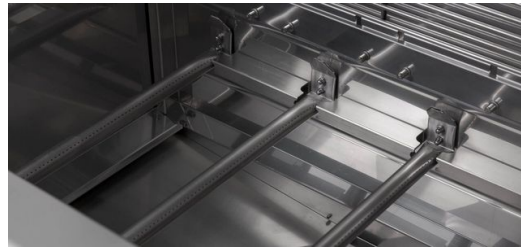
<p>The four stainless steel burner rods in the gas grills are cut on a TRUMPF laser tube cutting machine and each has 144 holes. The hole diameter, which becomes smaller towards the back, guarantees even heating of the entire grill grate.</p>
