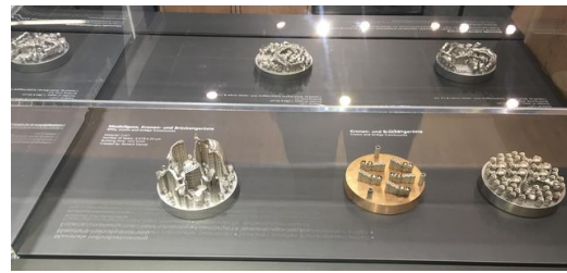
Substrate plates with 3D-printed dental prosthesis.
