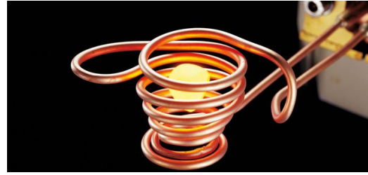
A coil envelops a fusion crucible. The material to be melted is put into the crucible and heated. Alternating current flowing through the coil, generates an electromagnetic field which transfers the electrical energy to the melting stock in a non-contact manner. (Image: TRUMPF)
