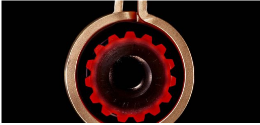
Inductive hardening of a gear part: Like the laser, induction is extremely local. Good conditions for efficient cooperation in flexible process chains. (Image: TRUMPF)
