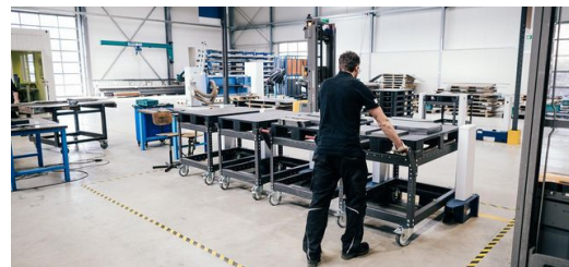
Sensors at the docking station detect when a pallet or pallet cage is parked and report this directly to TRUMPF's TruTops Fab software, which then takes over the automatic transport control. (Foto: Cornelius Bierer)
