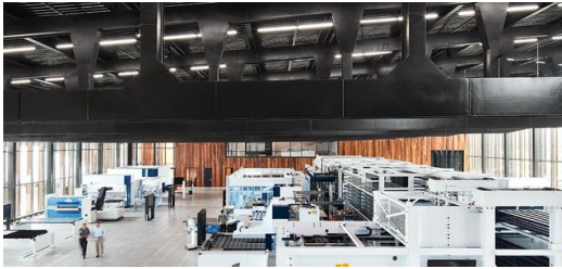
In a production hall measuring 55 meters in length, there is a connected sheet metal production with a central storage system as the centerpiece, which supplies the machine tools with material. Picture: Steve Hall © Hall+Merrick
