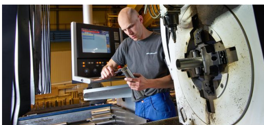
Each day one or two of the programmers are fully occupied with preparations for two-shift operations. The TruTops Tube Software makes possible exact calculation of cutting geometries. Picture: Escherich
