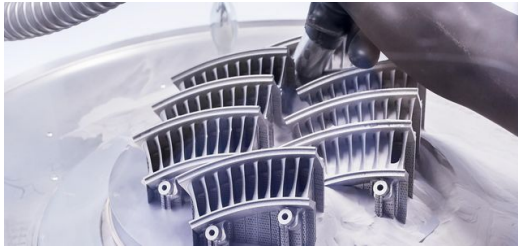
It takes just a few minutes to vacuum the excess powder off the part. (© Claus Morgenstern)
