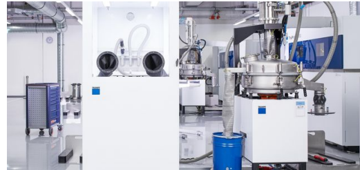
The excess powder is channeled from the unpacking station (left) to the sieving station. This unit cleans the excess powder so that it can be reused. It does this by removing the smoke residue and dirt particles picked up by the powder during the welding process. (© Claus Morgenstern)
