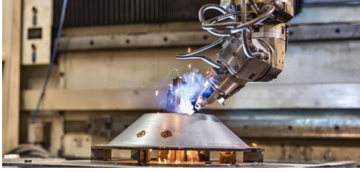
ELFIM uses the Lasercell 1005 for various applications of laser technology such as 2D and 3D cutting or welding and also for laser metal deposition. Picture: Antonio & Roberto Tartaglione
