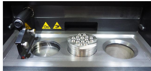
Preforms in TruPrint 1000: A fixture holding preforms in the 3D printer's build chamber
