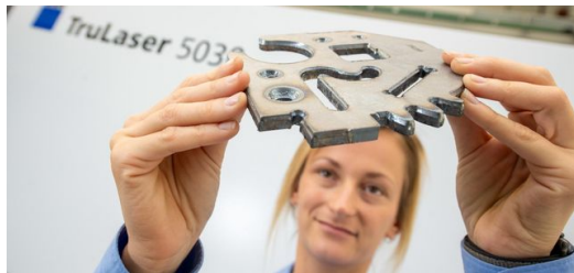
A worker checks a component she has chamfered using TRUMPF's EdgeLine Bevel technology.
