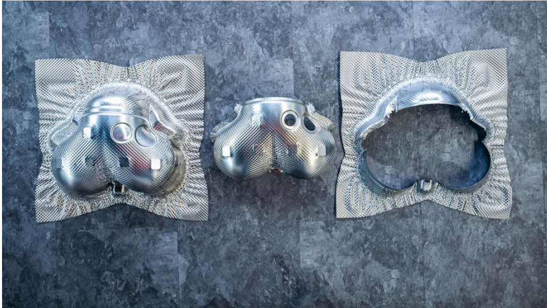
Deep-drawn form for a stainless steel outer shell (left), the 3D laser-cut final form (center) and overhang following removal (right).
