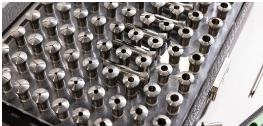
<p>Thanks to robust and flexible tooling setting up the machine with new part holding and aligning the optics takes less than five minutes: Here are the clamping devices for machine retooling.</p></p>
