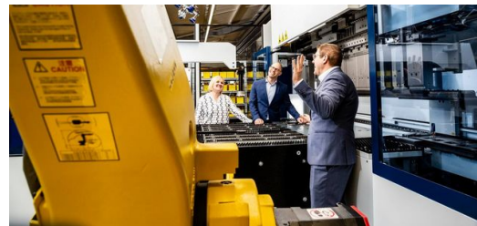
The Starmatik robot automation system for loading and unloading the TruBend Center 7020 speeds up production.
