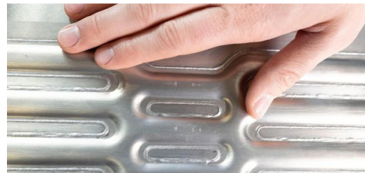
In the folding-box concept developed by BENTELER for a stainless steel battery housing, the patented TRUMPF solution BrightLine Weld ensures spatter-free processing and high-strength gas- and helium-tight weld seams, even in rapid series production.
