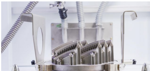
Done and dusted! A finished part from the 3D printer. (© Clauss Morgenstern)
