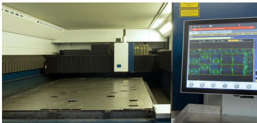
Programming with Smart Collision Prevention is simple and provides the highest degree of reliability, especially when cutting sheets under five millimeters thick. (Pototo Diez)
