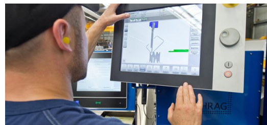
The machine's control system has a high-resolution, 17-inch color flat panel display with built-in touchscreen. This enables users to load 2D and 3D programs as well as 3D simulations. "The new control system is a bit like using a smartphone or tablet, so it appeals to our young machine operators," says Ingo Kleinau. Picture: Dirk Egelkamp
