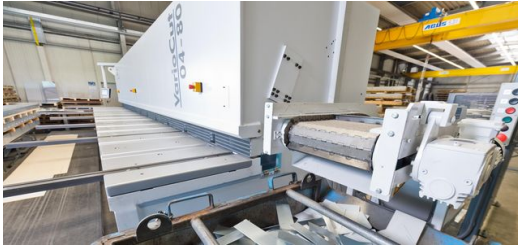
A scrap cutting system connected to the EHT VarioCut slices up scrap into small pieces. Picture: Dirk Egelkamp
