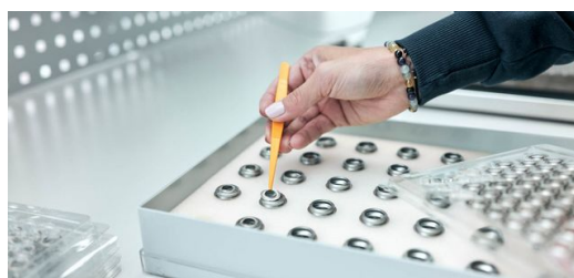
Preparation for the welding process: Placing the lenses on the stainless-steel sleeves is still manual work.
