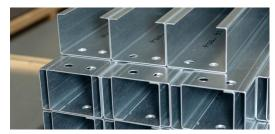
recise product analyses by the SCHRAG project group show that some profiles exhibit a certain degree of standardization. In the future, these profiles will be produced automatically on a roll forming line at SCHRAG's Hamburg Seevetal site.
