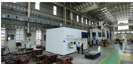
Originally bought for prototyping, JBM is using the TruLaser Cell 7040 now to process parts made of high strength steel.
