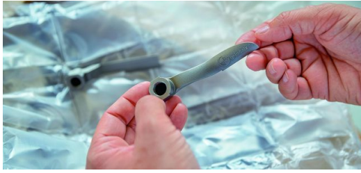
All one piece: Redesigned by Bionic Production, this nozzle offers gentle curves straight from the 3D printer. Picture: Claus Langer
