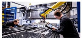
Autz + Herrmann mainly processes thin sheet metal. The low-pressure suction cups of the Starmatik robot automation system pick up blanks very gently.
