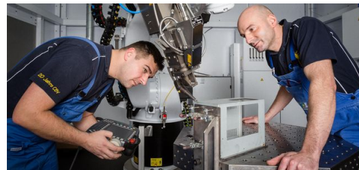
Daniel Voss, a welder at CBV, and design mechanic Marcus Hüttenrauch found their own ways to get the best from the TruLaser Robot, after a training session at TRUMPF. They shorten set-up times and costs by manually tracing the components in advance with the robot.
