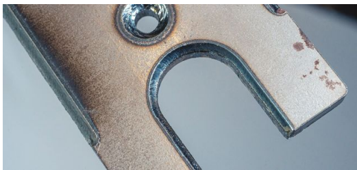
The technology is hugely helpful with thick sheets: EdgeLine Bevel can process sheets up to eight millimeters thick.
