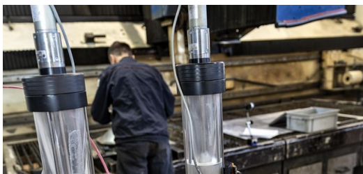
In combination with a powder feeder, the Lasercell 1005 from TRUMPF is also highly suitable for laser metal deposition. Picture: Antonio & Roberto Tartaglione
