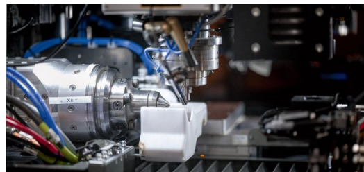
The principle of laser rotation: (to the left) the air-bearing rotational axis that holds the workpiece; the trepanning unit works from above. The workpiece rotates at a speed of 3,500 rotations per minute, where the focus circles are 30,000 times per minute.
