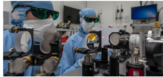
<p><span lang="EN-US">Mirror assembly in the TRUMPF clean room for production of the EUV laser system.</span></p> – TRUMPF
