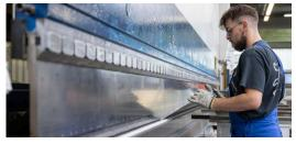
Automation reaches its limits in the production of special profiles. At SCHRAG, they will continue to be processed by bending professionals on bending presses. At SCHRAG's Hamburg Seevetal location, a 12.5-meter press from TRUMPF completes the existing press line.
