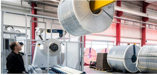
Machine operator Martin Müller heaves a 16-ton aluminum coil into the loading zone of the TRUMPF TruLaser 8000 Coil Edition.
