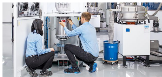
The construction cylinder is mounted in the unpacking station. (© Claus Morgenstern)
