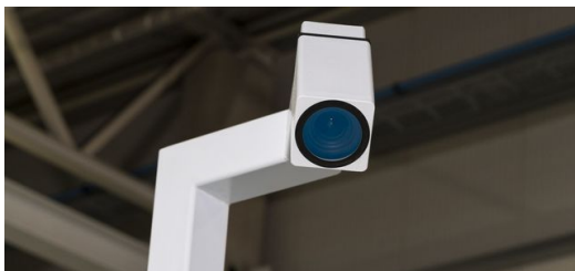
A high-resolution camera captures every part that is removed. The intelligent image processing of the Sorting Guide reliably detects it and reports the removal to the TruTops Fab production control.
