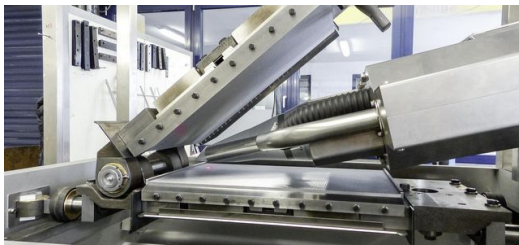
Despite the lack of space between the baking plates, the laser cleans them quickly and reliably. Picture: Maria Haas
