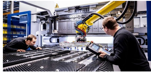
Autz + Herrmann mainly processes thin sheet metal. The low-pressure suction cups of the Starmatik robot automation system pick up blanks very gently.
