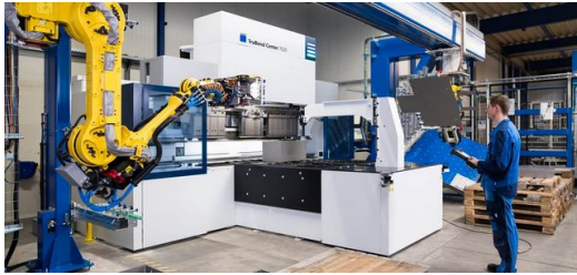
<p>The new TruBend Center 7020 panel bender made production of the field stove possible in the first place. Only with this equipment was the team at Kuipers able to automatically bend the relatively large firebox of 333 millimeters. </p>
