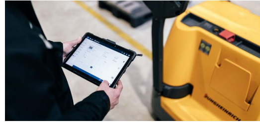
With the help of the intuitive interface of TruTops Fab Logistic, workers can check orders in and out using tablets, even on the shop floor. When an order is reported as completed, TruTops Fab automatically generates a transport order for the automated guided vehicle system. (Foto: Cornelius Bierer)
