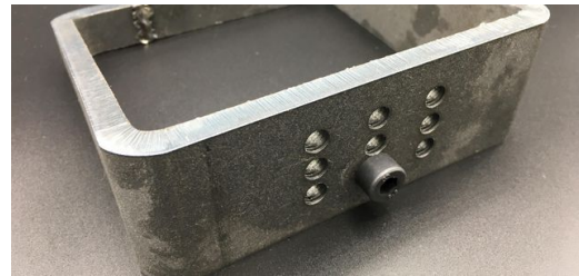
<p>The TruLaser Tube 7000 can be used to fabricate a range of different threads in tubes.</p>
