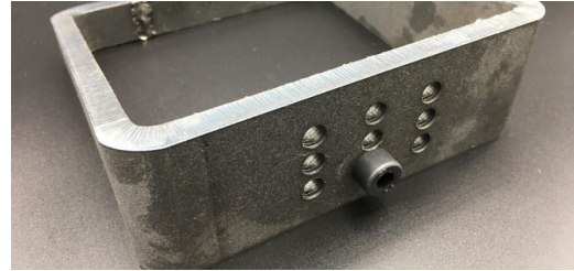
The TruLaser Tube 7000 can be used to fabricate a range of different threads in tubes.
