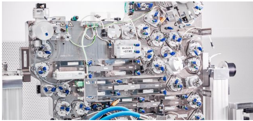
Mirror support on a EUV-module
