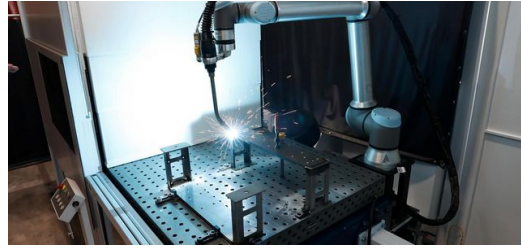
The automated welding cell that is easy to program, has many parameters already integrated and at the same time meets high quality standards: the TruArcWeld 1000 from TRUMPF.
