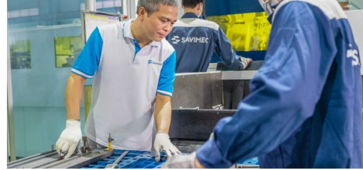
Processing accuracy is important to Ngo Sach Vinh: “We process square, round and oval tubes with different diameters. The setup-free self-centering collet chuck of the TruLaser Tube 5000 fiber automatically ensures that the tubes are correctly clamped into the machine.”
