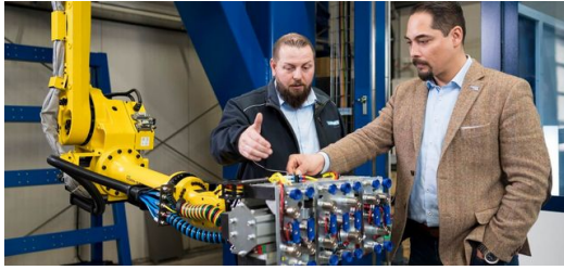
Just in time, the robot automation for loading and unloading the TruBend Center 7020 was also put into operation. "This adds speed to the production process," said Michael Kuipers (right), and Karsten Hanenkamp added, "The grippers place finished parts on waiting pallets for further transport to the welding shop."
