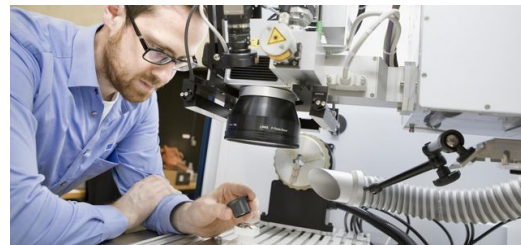
<p><span lang="EN-US">For the engraving of the platinum watch backs, TRUMPF machine operator Matthias Widmer very carefully approached the desired engraving depth of 17 micrometers.</span></p>
