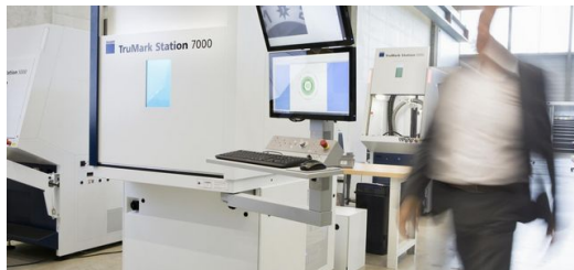
<p><span lang="EN-US">The edition engraving for the Meister S Chronoscope Platinum Edition 160 was created in a TruMark Station 7000 equipped with the new generation TruMicro Mark Series 2000 ultrashort pulse laser.</span></p>
