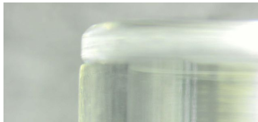
Lateral view: Laser-welded protective caps are more than twice as strong as conventionally joined caps in breakage tests.
