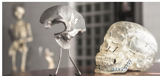
<p>What the eye can’t see: the surfaces 3D printing can produce are the key to promoting a connection between the bone and the implant.</p>
