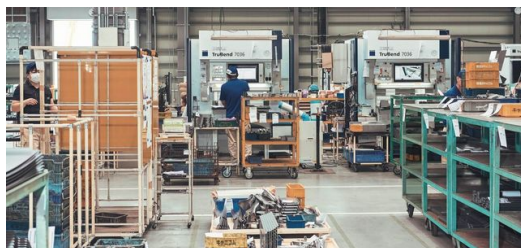
The meticulously planned layout of the new production facility and the configuration of the TRUMPF machines has reduced production time by 40 percent.
