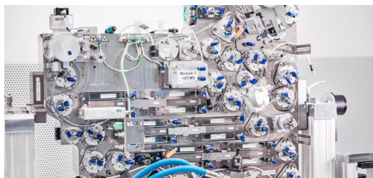
Mirror support on a EUV-module
