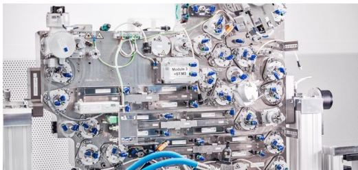
Mirror support on a EUV-module
