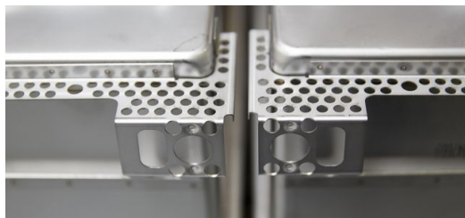
Formed areas – like brackets, threads and hinges – are now made up quickly and easily on the TruMatic 6000 fiber. (Picture: Claus Langer)
