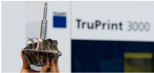
At EMO 2019 TRUMPF showed a 3D printed gas compressor made from Inconel. Time savings: 50 percent.
