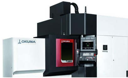
The multifunctional machines of the LASER EX series combine subtractive and additive manufacturing and enable the hardening and coating of workpiece blanks.
